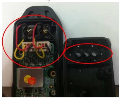
Step 10. Mounted on the back cover and check the wire is exposed in the hole bits.
