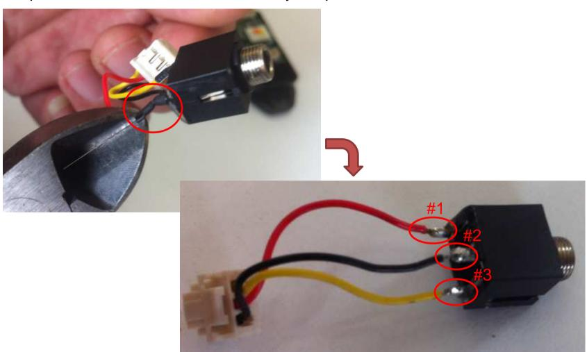
Step 6. De-soldering the earphone connects cable by soldering Tools
