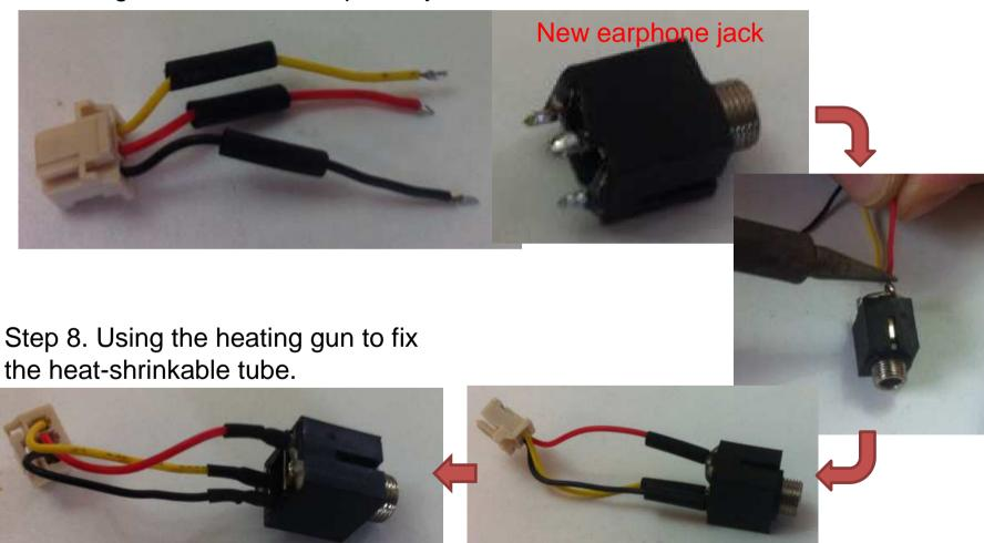
Step 9. Finishing the wire cable to avoid installing interference
