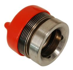
This shaft seal uses a carbon ring in the bellows assembly, and a silicon carbide stationary ring in the seal plate. These are the same proven materials that are used in Carrier compressors today.
