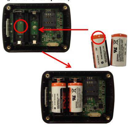
Figure 6. Backup Battery Installation
