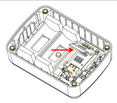
Figure 5. SIM Card Installation
