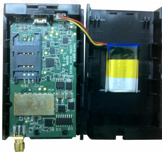
Figure 6. Backup Battery Installation
