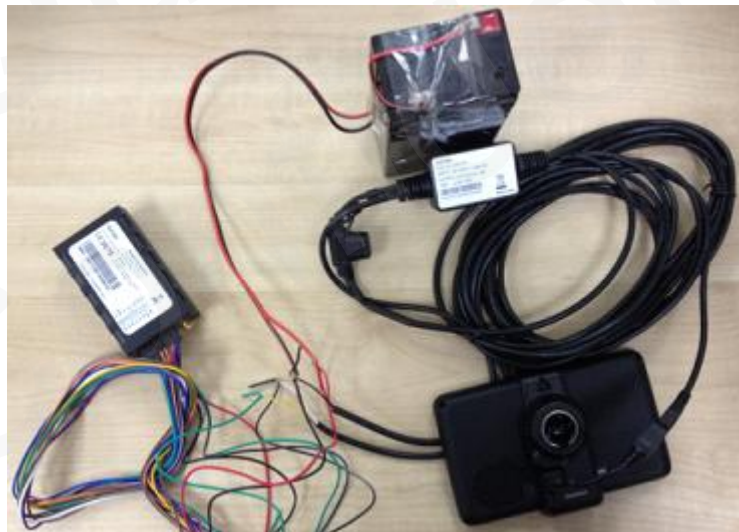
Figure 18. GV300 connection with Garmin GPS set
