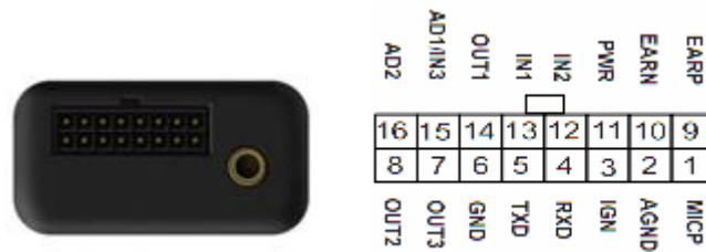
Figure 2. The 16 PIN connector on the GV300
