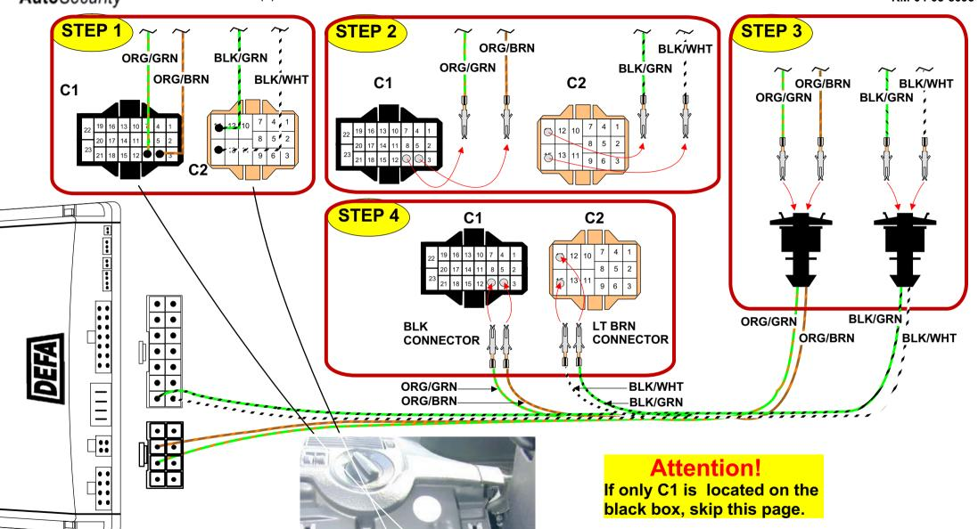
Attention! This installation diagram must only be used as a guideline for the installation. Equipment delivered with the car varies considerably from model to model and from market to market. Before starting the installation, be sure to check carefully the original diagram from the car manufacturer. DEFA A.S is not liable to compensate for possible damages that may occur due to faulty or insufficient installation manuals
