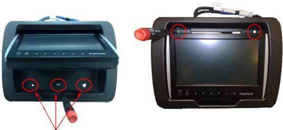
Picture 7 – Fixing of holder with screws
