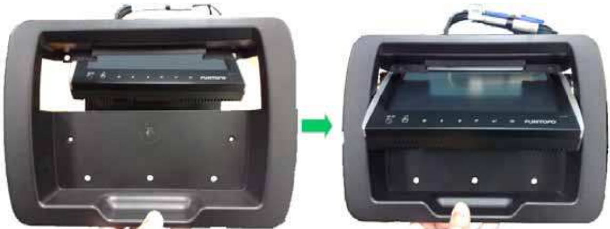
Picture 6 – Installation of the holder
