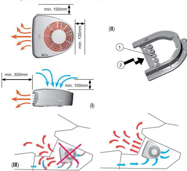
The interior heater must be installed in such a way, that it does not pose a safety hazard in case of an accident or abrupt braking. When drilling holes and installing screws to mount the holder, always make sure that no cables or time-program controllers on the back of the wall will be damaged.
